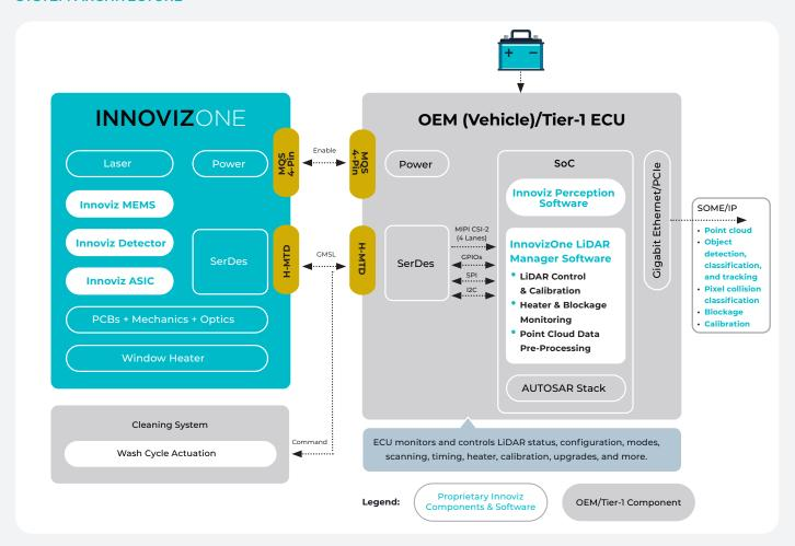
InnovizOne data packets must be converted to the format used by the OEM's perception software. This packet format conversion can be done in an external component or directly in the OEM's ECU.
